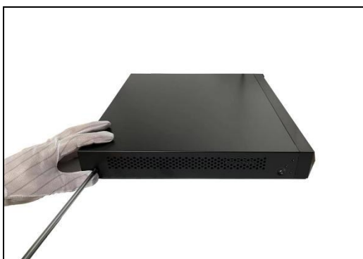
Figure 1-11 Install the cover and screws
