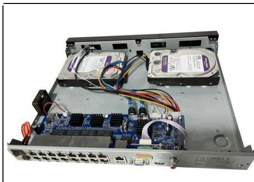
Figure 1-9 Connect the power and data cables
