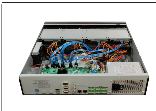
Figure 1-13 Connect the power and data cables
