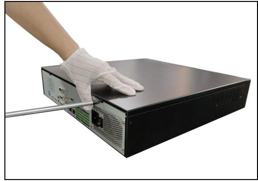
Figure 1-15 Install the cover and screws
